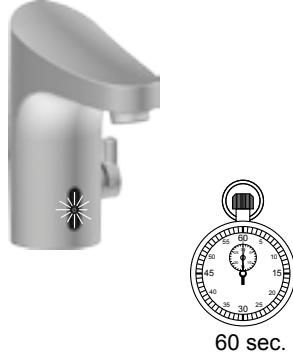
**EN** - Start the mixer once before activating this function. Press and keep your finger on the lower part of the sensor window for one second to start a 30 second flush cycle. To cancel the flushing, put your finger back for two seconds.
